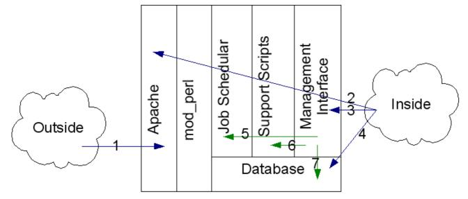
In the above diagram, "Outside" refers to any customer connectivity to the system (where a customer can be a person or application) and "Inside" refers to the developpers and administrators of the LAMPAS system.
